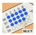
3. Remove. Wait approximately 10 seconds. Some blue dots may disappear as device "locks in" for accuracy. Read temperature indicated by last blue dot.
