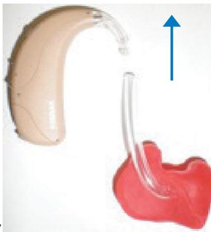
tubing on to the elbow of the aid, as shown.
