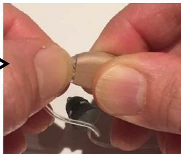
Then pull firmly to remove the tube from the aid.
