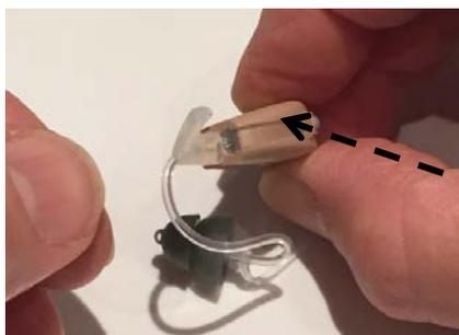
Then twist the top of the tube anticlockwise 90 degrees so it looks like this:
