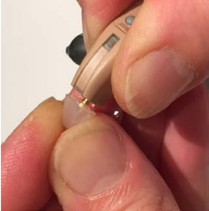
Then reconnect the tube by firmly pushing the triangular end straight back on to the aid – it should click on.
