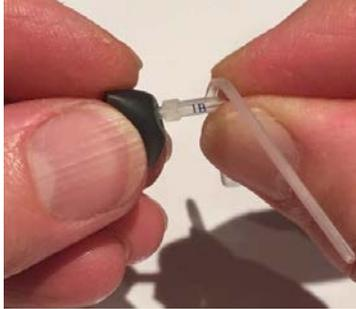
Then, take the wire and thread it through the tube from the triangular end towards the narrow end where the dome was.
